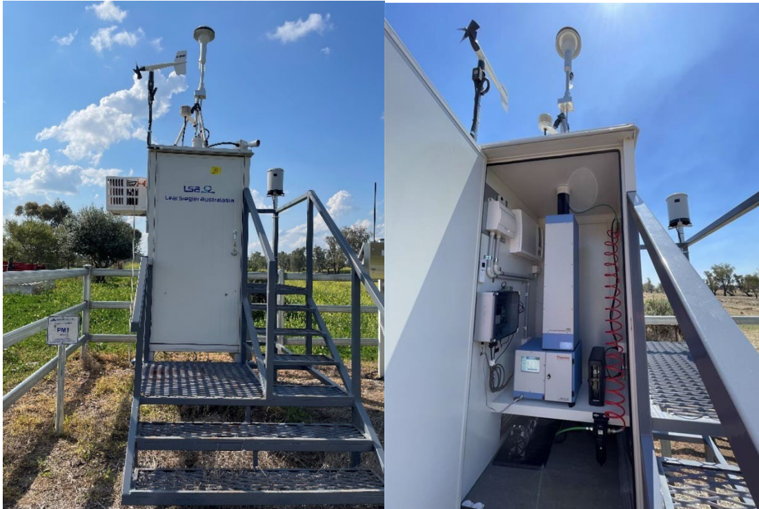
Figure 1: TEOM installed at Lanreef
